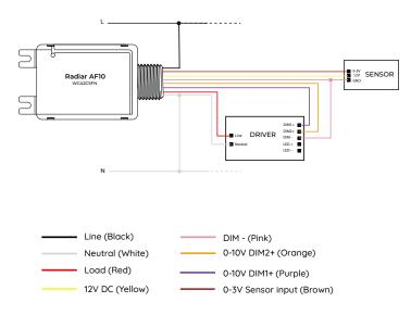
2. Configuring Radiar AF10 for dimming, tuning and an external sensor control (with additional surge protection)
